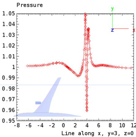
Figure 2. Example of pressure versus line plot along a line  $y=3, z=0$  (blue line).
