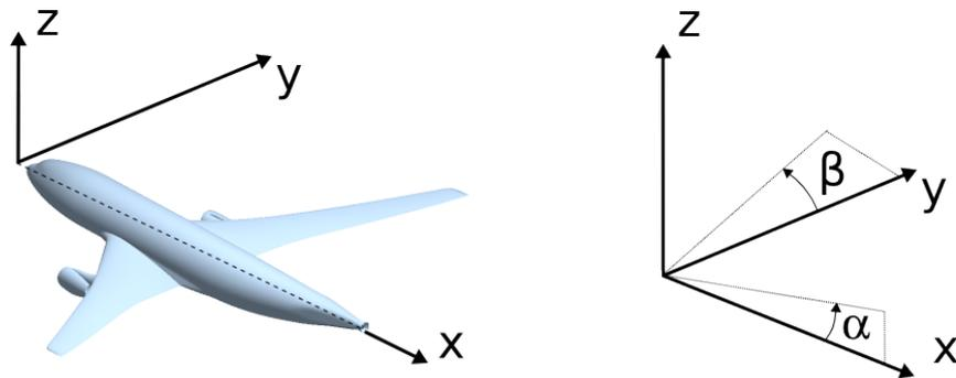
Figure 4. CFDxy plot model axes (left) and definition of pitch angle  $\alpha$  and yaw angle  $\beta$  (right).
