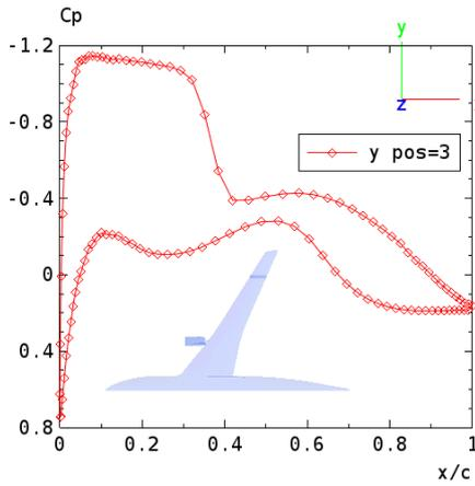
Figure 1. Example of wing profile  $C_p$  plot at position  $y=3$ .
